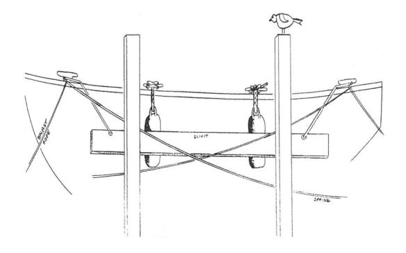
**Alternative Fendering**: Fix solid rubber fendering to the staging's uprights. (Rope, carpet, etc, doesn't last long.) This is by far the best method in the long run.
